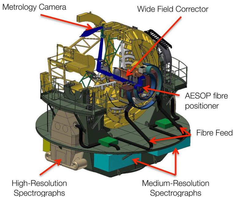
Figure 6: A schematic of ESO's VISTA telescope and the 4MOST re-fit including AESOP
