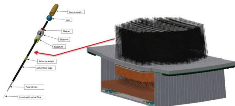
Figure 7: A schematic showing the AESOP Echidna layout (right) and a zoom in on an individual Echidna spine (left).
