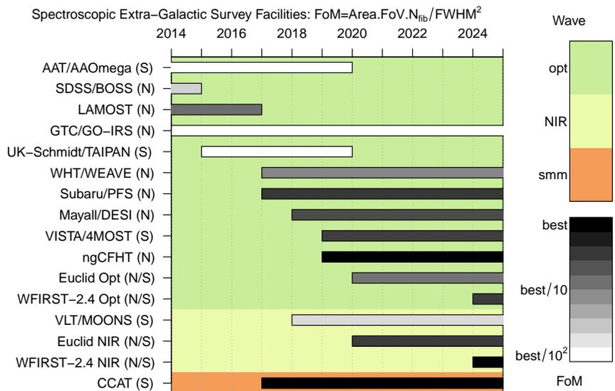
Figure 5: A graphic comparing wide-field spectroscopic facilities using a standard figure-of-merit (FoM). The greyscale of the bars relates to the FoM with black representing the best and white the worst on a logarithmic scale. While Australia has a fairly unique hold in this area the facilities under development, which rely on Australian built components, will soon out-compete Australia’s capacity in this area.
